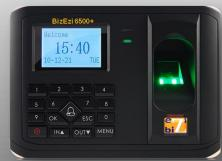
The BizEzi WS6500+, is a professional biometric fingerprint reader used for time and access control.
